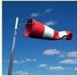
Wind sock (Speed and wind direction)
